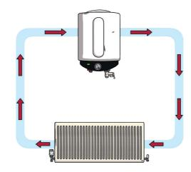
In the boiler and radiator model, the pump pushes the water around the system. It does a similar job to a **battery** Resistance is measured in **ohms**  $(\Omega)$ . pushing the **charges** around a circuit. The pipes carry the flow of water around the system, like the **charge** flowing Resistance can be calculated using the equation: through wires in a circuit. The radiator is similar to a bulb because it transfers **energy** supplied by the system to the surroundings.
