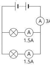
The current is split between the branches in a parallel circuit.
